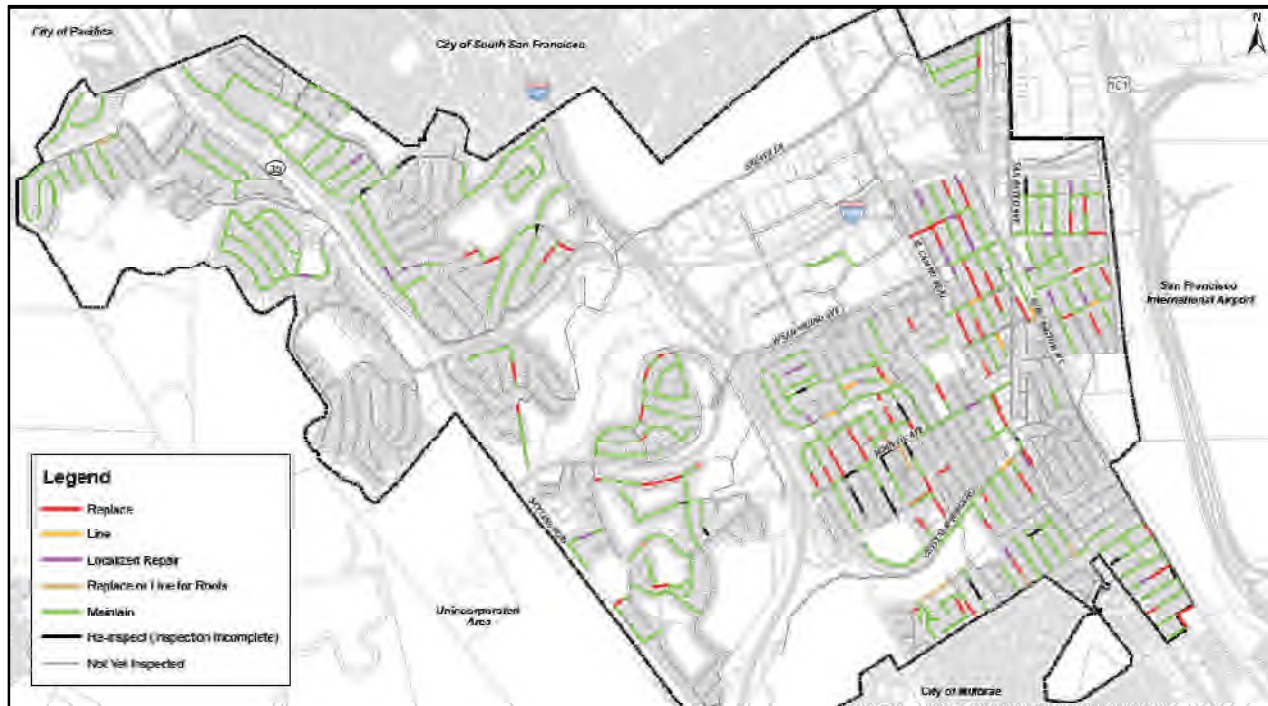
Figure 1: Sample Pipeline Condition Assessment Map
